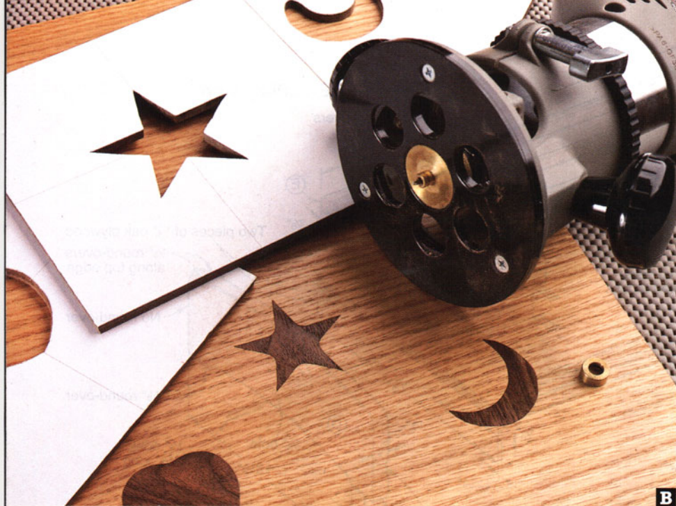
C A router inlay set ( above ) consists of a precision inlay bushing, a bushing retaining nut, a bit-centering pin, a \frac{1}{8} " downcut spiral bit, and a \frac{9}{16} "-diameter collar.
